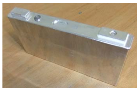
Figure 4: Li-Ion prismatic hard case cell design (ZSW-manufacturing, 2015)
